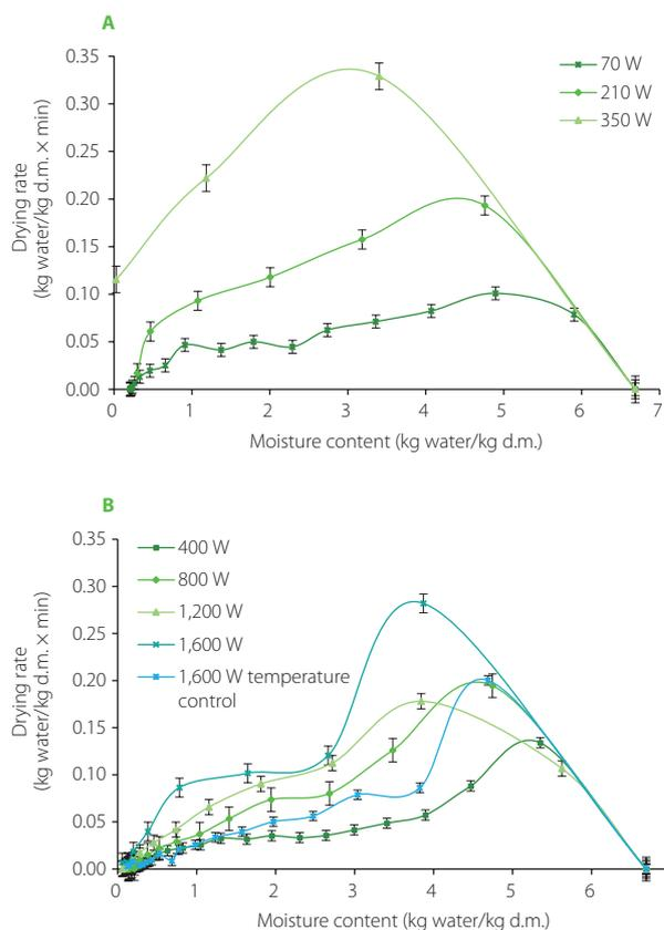
**Figure 2.** Curves of drying rate versus moisture content of the apple cubes dried at different microwave powers in a rotary plate microwave dryer, RMD (A) and a microwave convection coupled dryer, MCD (B); d.m., dry matter.
