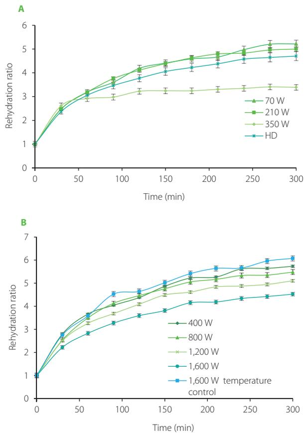
**Figure 5.** Rehydration ratio curves of the apple cubes dried at different microwave powers in a rotary plate microwave dryer, RMD (A) and a microwave convection coupled dryer, MCD (B) HD, hot air drying.
